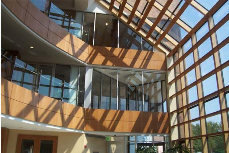
The lobby boasts a new South American hardwood finish. Renovations for this atrium cost over one million dollars. Gilbeaux Associates designed 16 tons of cooling furnished by new water source heat pumps to maintain comfort and humidity levels in the space year round.
